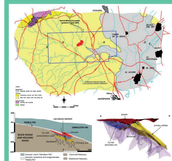
Location map and schematic geologic cross sections for the Las Cruces deposit. Source: Cobre Las Cruces Operation Technical Report NI 43-101(2015), Scheiber et al. (2018), Yesares et al. (2017).
