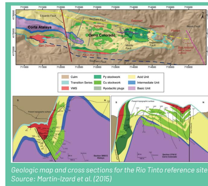
Geologic map and cross sections for the Rio Tinto reference site. Source: Martin-Izard et al. (2015)
